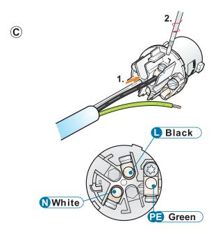
(C) Insert wires into terminals L, , PE and tighten.
