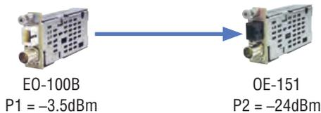
$$LB = -3.5\text{dBm} - (-24\text{dBm}) = 20.5\text{dB}$$
