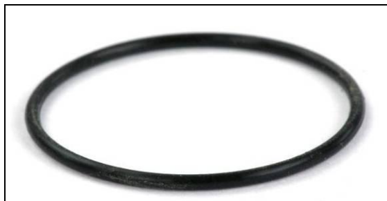
Fig. 9: O-ring after 5000 mating cycles
