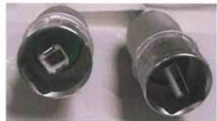
On the left: Small quantity of dust on the metal part
