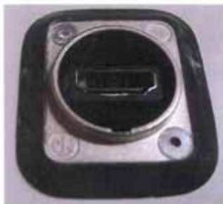
Small quantity of dust on the metal part
